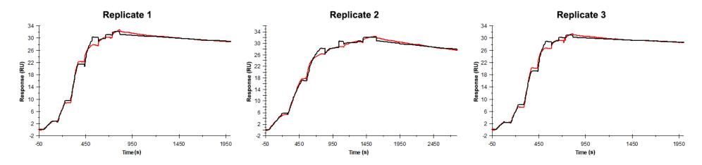
Sensorgrams obtained for each replicate of peptide  $3 / Phd_{STm}^{52-73}$  D53A (analyte) binding to Doc<sub>STm</sub> (ligand). Six concentrations of the analyte were flown over the surface in a single cycle, ranging from 50 nM to 0.206 nM (3-fold dilutions). The association times were 80s for replicates 1 and 2 and 200 s for replicate 3. In all replicates the dissociation time was 1200 s.
