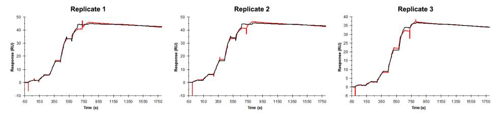
Sensorgrams obtained for each replicate of peptide 2 / Phd<sub>STm</sub><sup>52-73</sup> M52A (analyte) binding to Doc<sub>STm</sub> (ligand). Six concentrations of the analyte were flown over the surface in a single cycle, ranging from 100 nM to 0.412 nM (3-fold dilutions) for replicates 1 and 2, and 50 nM to 0.206 nM (3-fold dilutions) for replicate 3. The association and dissociation times were 80 s and 1000 s, respectively.
